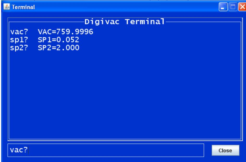
Press carriage return or enter to submit the query or change the set point. Note that while the web terminal is open, the main 200 Pirani screen will not update. If at any time the web terminal or the main 200 Pirani applet window becomes unresponsive, close the browser (not just reloading the tab or closing the tab) and reconnect.
