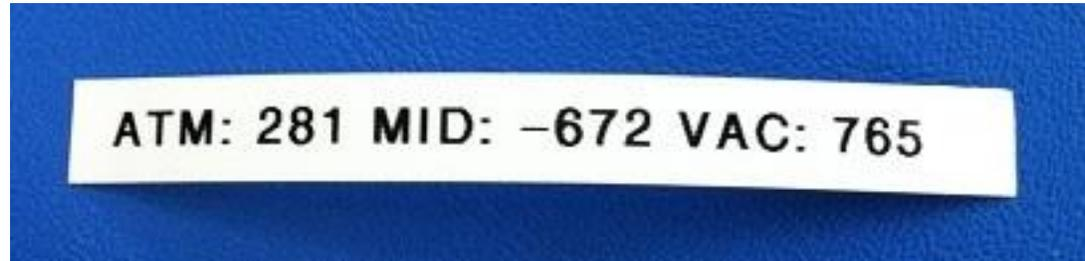
These numbers, or “offsets”, when entered correctly into the calibration menu, will automatically calibrate your BPG to the assigned tube without additional testing.
