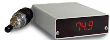
**PiezoTorr Manometer** | Measures from 1 Torr up to 760 Torr, similar to a 1000 Torr capacitance manometer and controller assembly. It is available in Torr or mbar.
