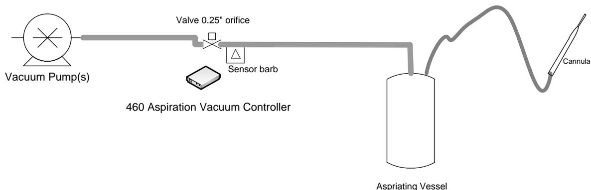
**RESULTS:** The DigiVac engineering team used an iterative approach to design and develop a product that met the specific needs of the client for consistent and precise vacuum regulation during the aspiration process.
