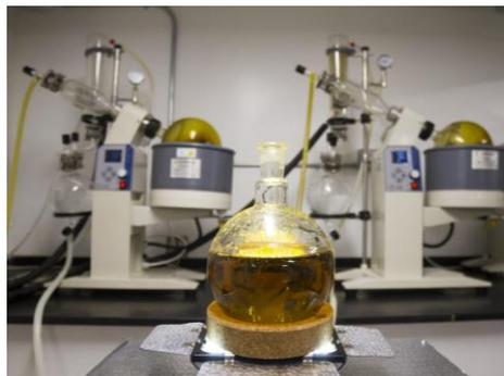
In rotary evaporation, you do not care what happens with the vapors of the solvent, but distillation setup is specifically built for collecting vapors, and even separating vapors of different compounds.
