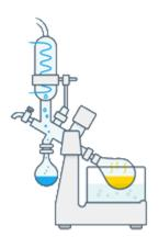
Rotary evaporation distillation, a form of low pressure vacuum distillation allows you to effectively separate components of a mixture and condense the final product to what is needed. For example, using distillation to separate water and alcohol so you have one glass of mostly water and another with mostly alcohol. Using vacuum to reduce pressure enables you to lower the temperature of distillation.
