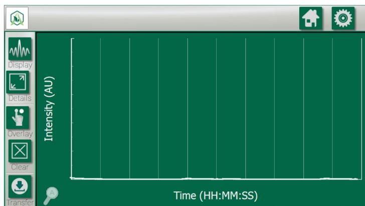
**What it does:** Displays and tracks the interpreted values from your measurement. This plot reduces the raw data and shows you the “highlights” of the run.
