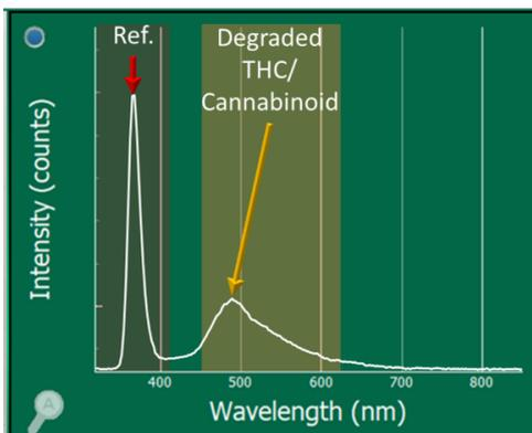
**TIP:** Degraded THC/cannabinoids are typically considered “undesirables” and should not be collected.
