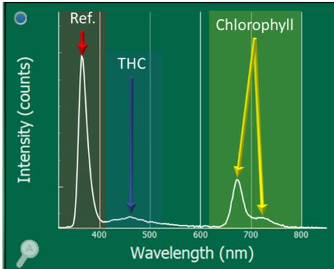
**TIP:** If a WFE operator sees the Chlorophyll signal, s/he should perform a carbon scrub (or other chlorophyll remediation) before starting distillation or on the distilled product. If Chlorophyll is detected on the distillate line of the cannabis refining pass, wiper speed should likely be increased or WFE internal chamber temperature decreased.
