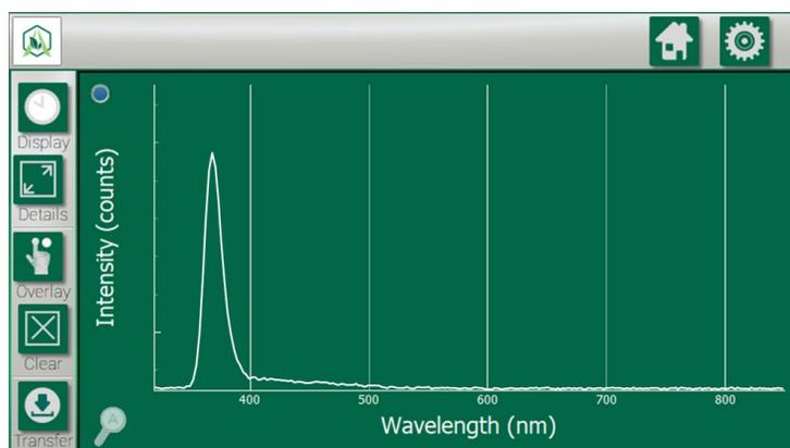
**What it does:** Displays current background/ambient light corrected spectral measurement.
