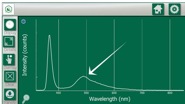
**Option B - Wavelength View:** This view will show that there is a sharp increase in the value of the wavelength plot. An example plot is shown below. This view is recommended for this change.
