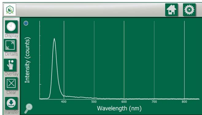
**Note:** The signal shown at 360-370 nm is the reference peak from the sensor’s light source. To remove this peak from view, press the blue “Reference Peak” remover button (available in 1.2.3.). Graph 2 below depicts what the Spectrum View looks like without the reference peak.
