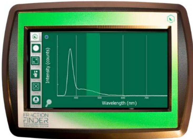
**TIP:** Similarly to CBD, Delta-9 THC is considered a “desirable” during WFE of THC. In these processes, the Fraction Finder can assist operators in collecting the most amount of this molecule as possible by indicating when it is passing through.
