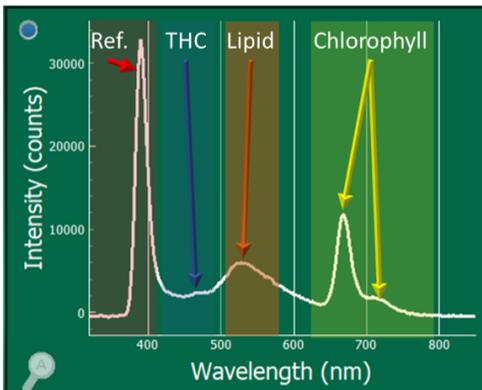
**TIP:** If a WFE operator sees the signal for Lipid (a peak that is centered between 530-620 nm), this indicates that their lipids removal is not removing all the fats.
